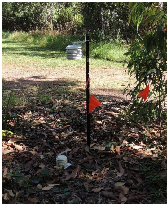
Figure 6. Solar shield setup with dataloggers in partial shade
