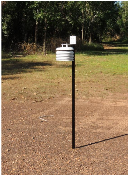
Figure 5. Solar shield setup in full sun (data logger inside shield at 1.2 m).
