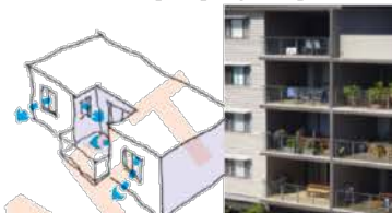
Articulated typical apartment with part-recessed balcony enables two rooms to capture breeze.
