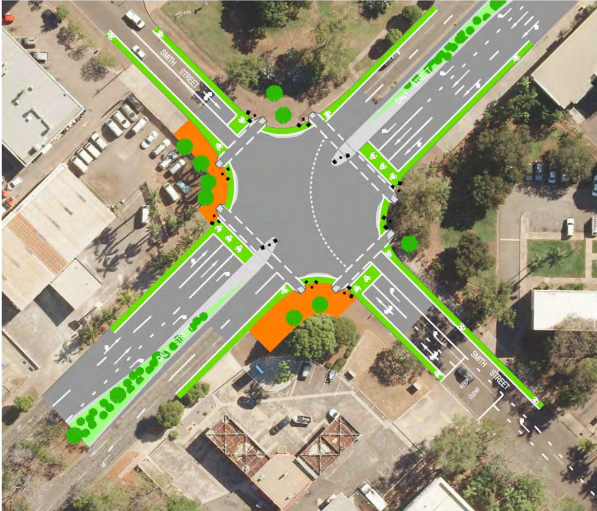
Figure 1. demonstrates the signalised intersection including future on road bike lanes, bike rider storage boxes and protected left hand turning lanes.
