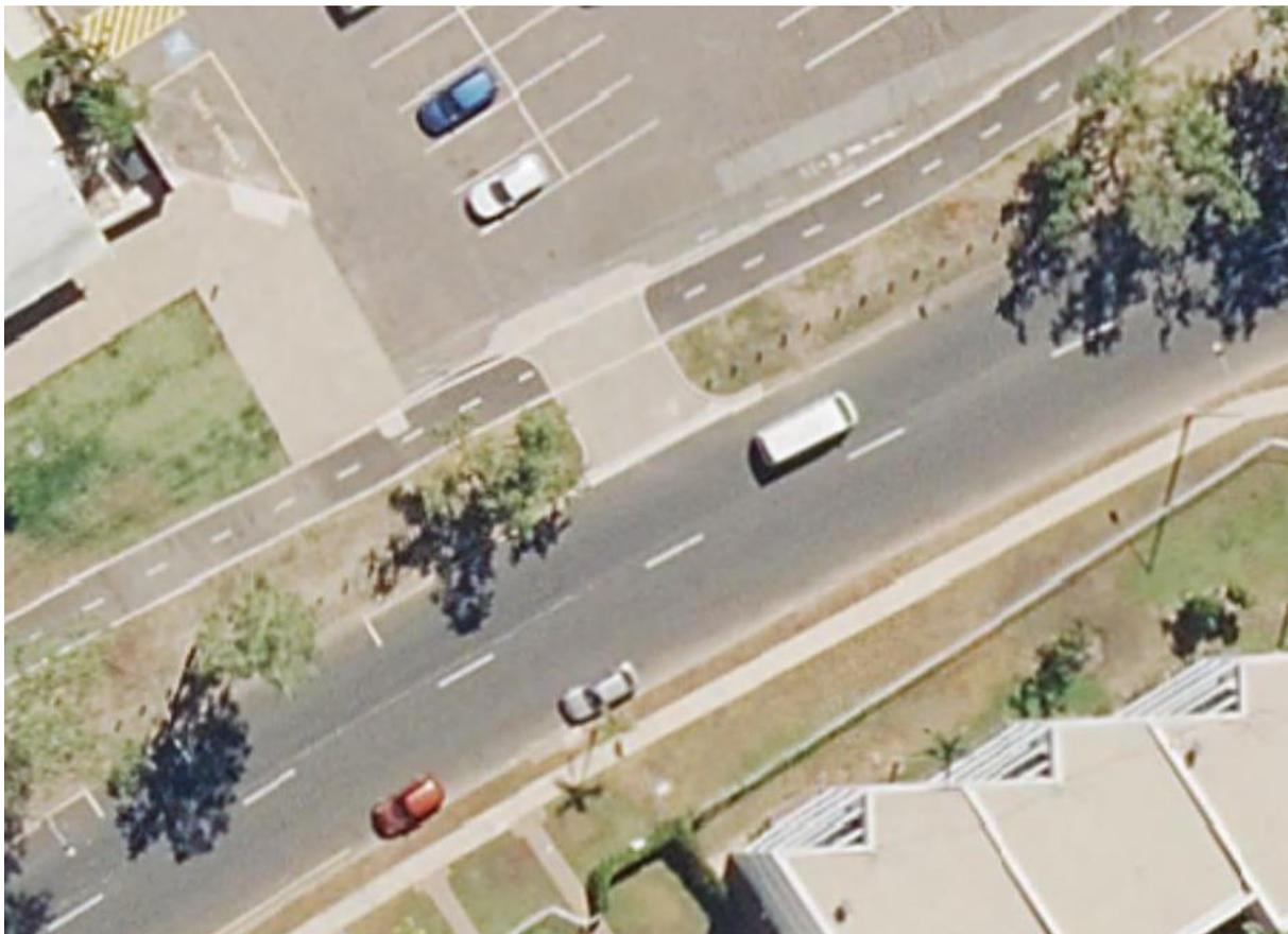
Where it is desired to give vehicular traffic priority at a driveway crossing, the crossover shall be constructed at the same level as the road carriageway with kerb ramps for path users. Give Way signs and markings shall also be used to clearly delineate priority.
