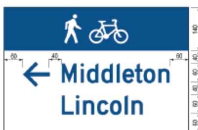
(d) DIP-2 Two-line direction indication sign artwork template
