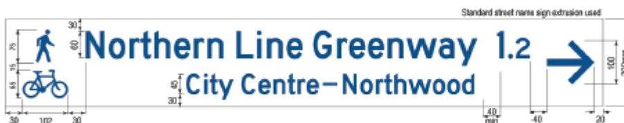
(c) FBL-2PR Local cycle route fingerboard indicating a junction with a primary route The end destinations of the primary route are shown on the lower line.
