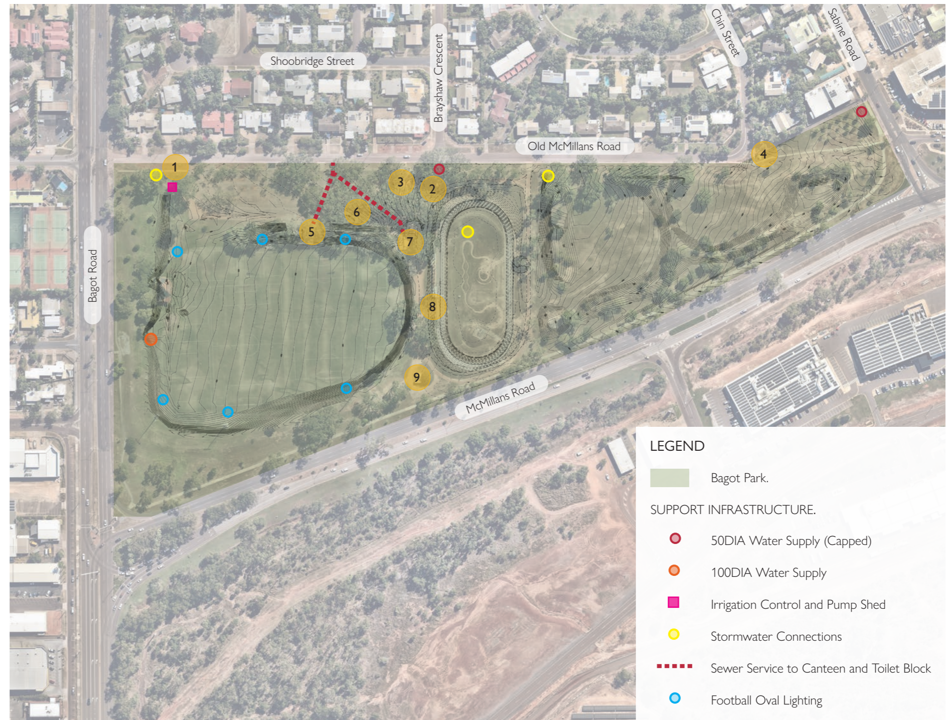
Figure 4.8 Existing Support Infrastructure at Bagot Park.
